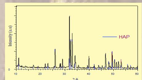
The X-ray diffraction patterns for HAP
