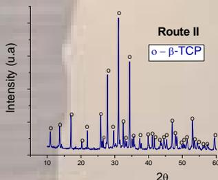
The X-ray diffraction patterns for  $\beta$ -TCP
