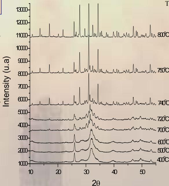
XRD patterns showing the transformation of apatitic tricalcium phosphate to crystalline  $\beta$ -TCP that occurs at a temperature between  $700 - 800^\circ\text{C}$ .
